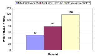
This kind of tribological stress during the tests corresponds to the particle erosion (erosion wear, abrasion) according to DIN 50320
