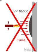
Irrespective whether the VP 10-500 has been applied to cold or warm metal, the metal temperature must not exceed approx. 130-150 °C up to the start of the curing process. If there is no suitable temperature measuring device available, we recommend the use of the self adhesive temperature indicators, which can be ordered at MultiMetall.
