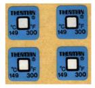
These are self adhesive one-way measuring temperature indicators, self temperature measuring points, which do change their colour from white to black after reaching the temperature printed on them (149 °C). Before applying VP 10-500, the temperature indicators must be removed i.e. using a spatula to achieve a good bonding of VP 10-500 on the surface.
