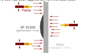
**Wrong!** The direct contact of the flame with VP 10-500 must be avoided.
