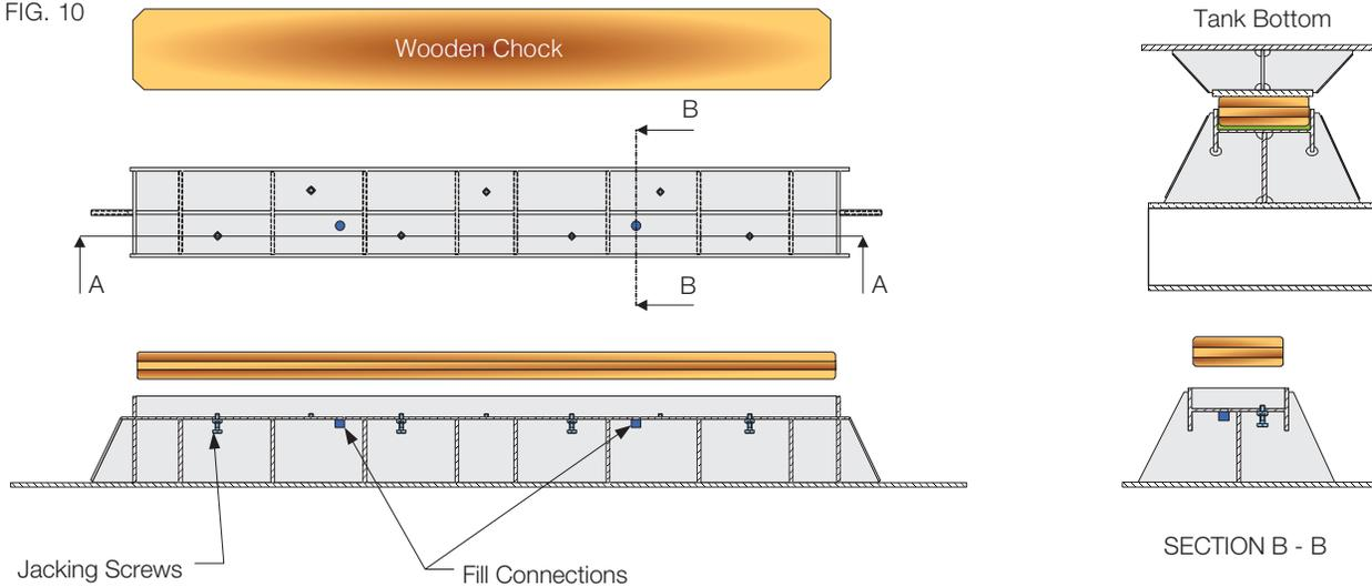
A positive displacement pump is connected through a series of hose with quick connect fittings, valves, and pipe fittings to the fill connections located under each support block. TG-7B is mixed and pumped into the void space at the bottom and around the sides of the block until it comes out around the top. After the mastic has hardened, the jacking screws must be removed.
