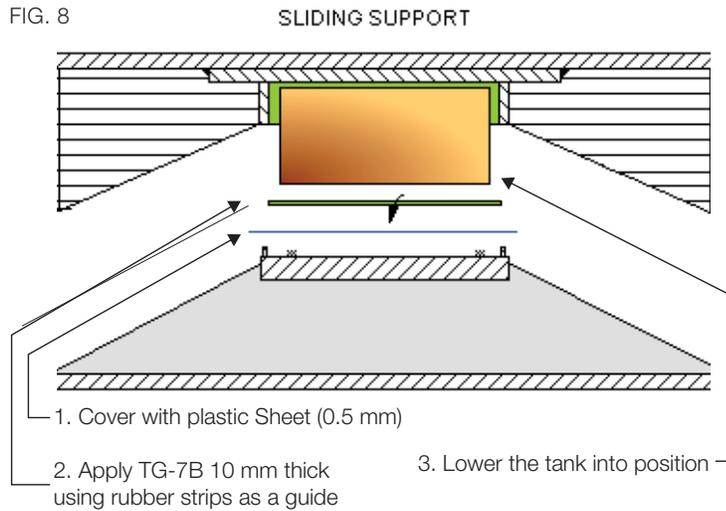
Sliding supports must be constructed in such a way that they are free to move as the tank expands and contracts. One way to do this is to apply TG-7B to the saddle and cover it with a non-stick plastic sheet. In this way, the mastic will adhere tightly to the saddle and conform to the exact shape of wood blocks but not stick to them.
