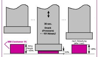
This is an evidence for the extraordinary positive compressive set of MM-Elastomer 95.
